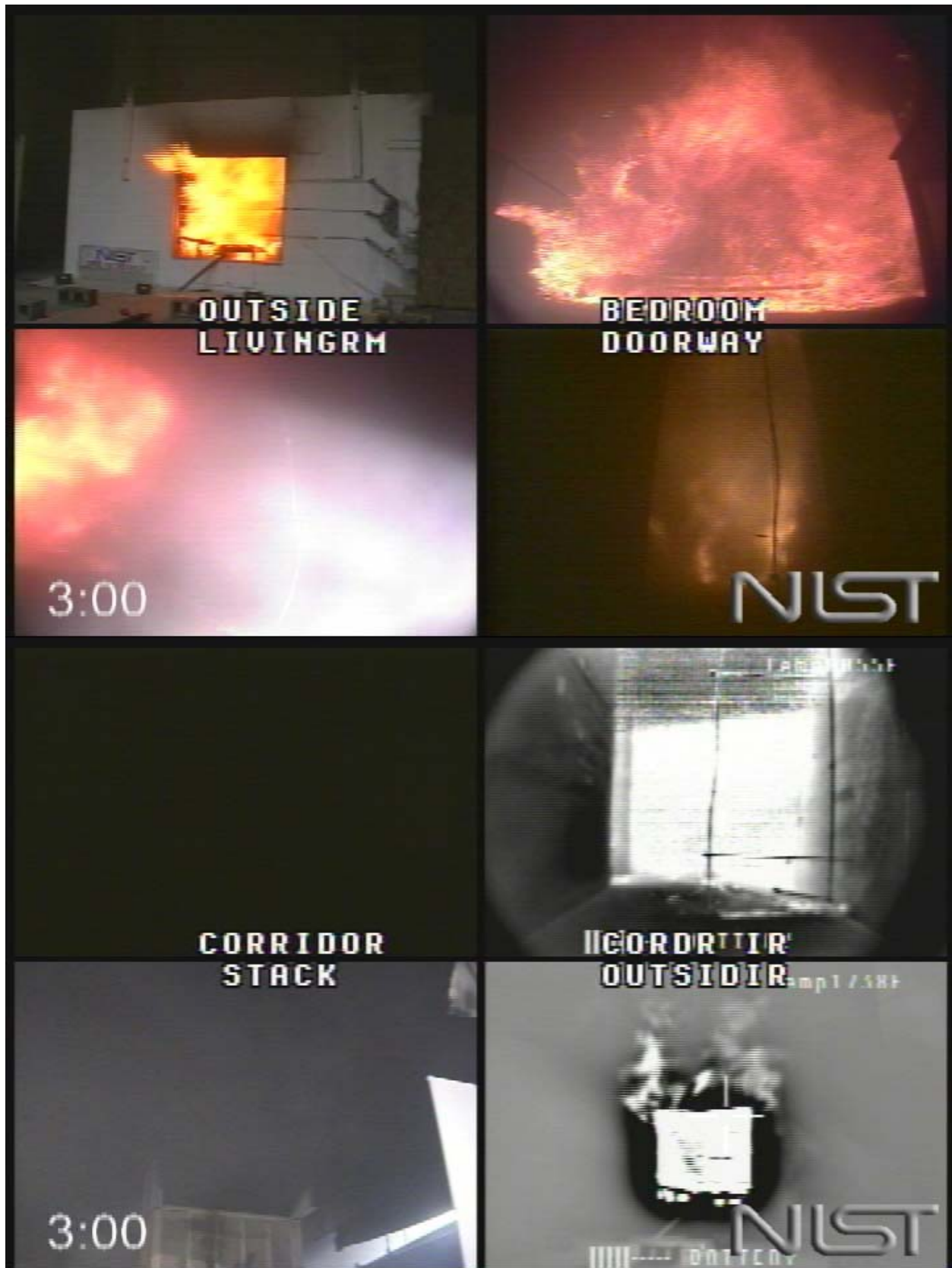
Figure 5.8.1-5. Experiment 8, 180 s after ignition.
