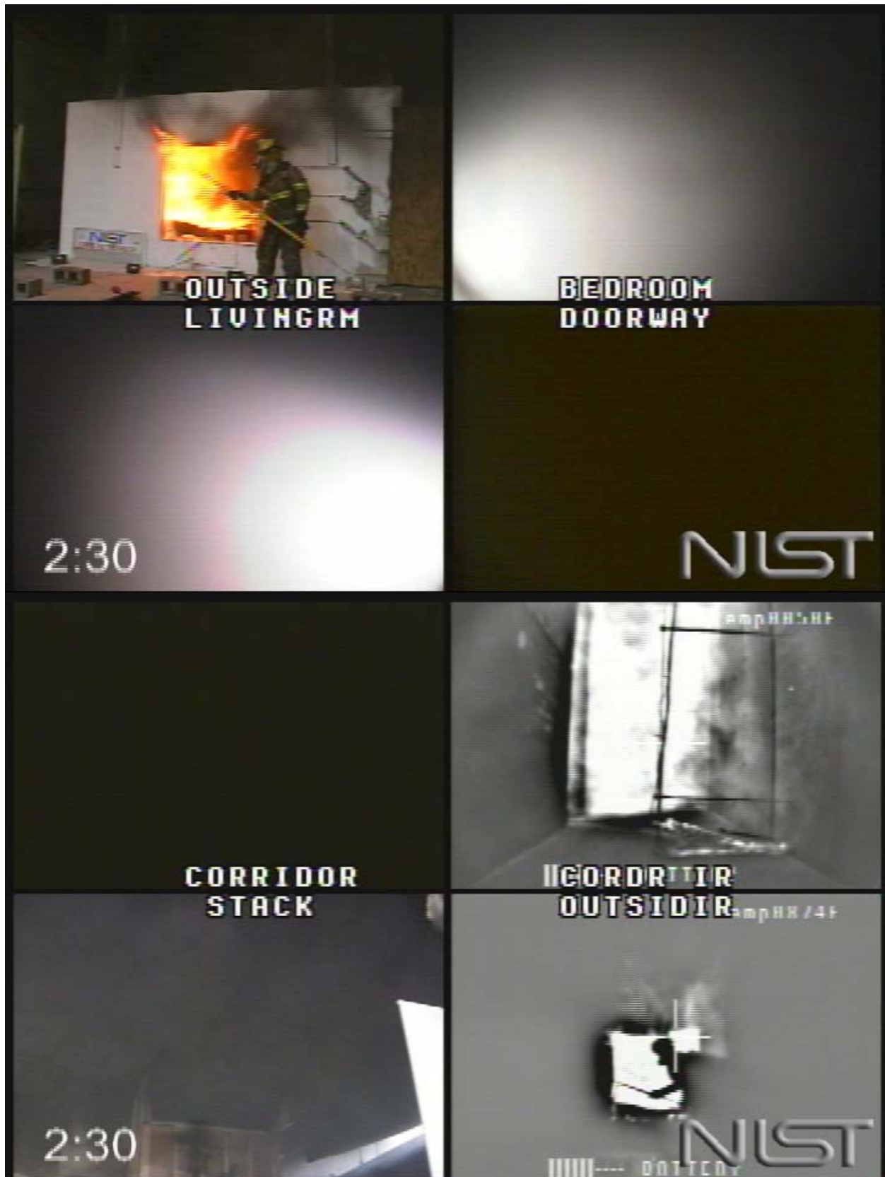
Figure 5.8.1-4. Experiment 8, window fully vented, 150 s after ignition.
