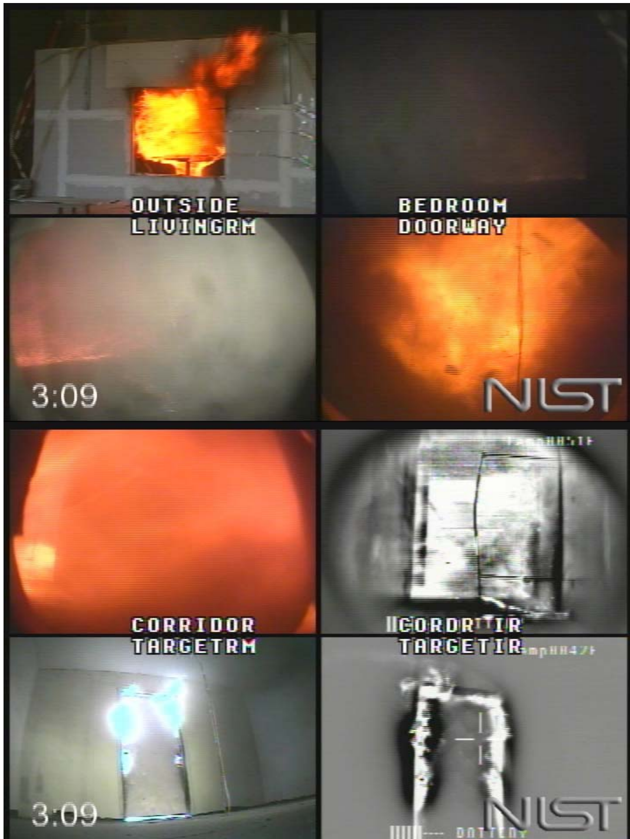
Figure 5.2.1-5. Experiment 2, corridor flames, 189 s after ignition.
