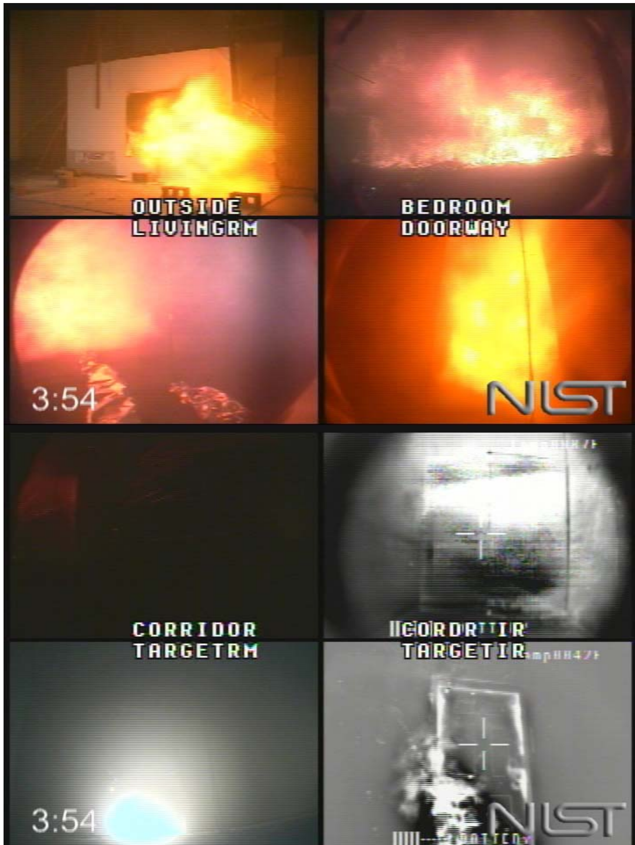
Figure 5.4.1-6. Experiment 4, corridor flames, 234 s after ignition.
