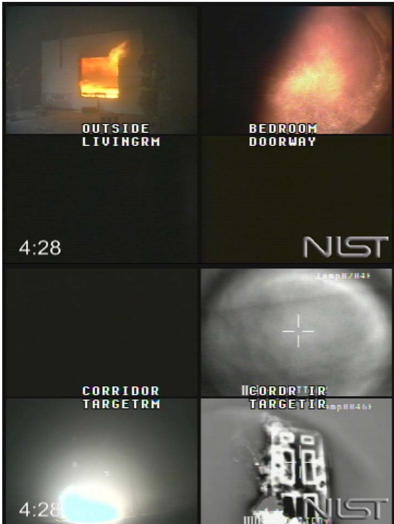
Figure 5.4.1-8. Experiment 4, 268 s after ignition, just prior to WCD deployment.
