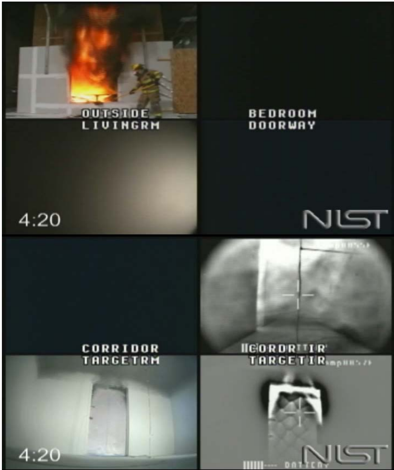
Figure 5.1.1-6. Experiment 1, window fully vented, 260 s after ignition.
