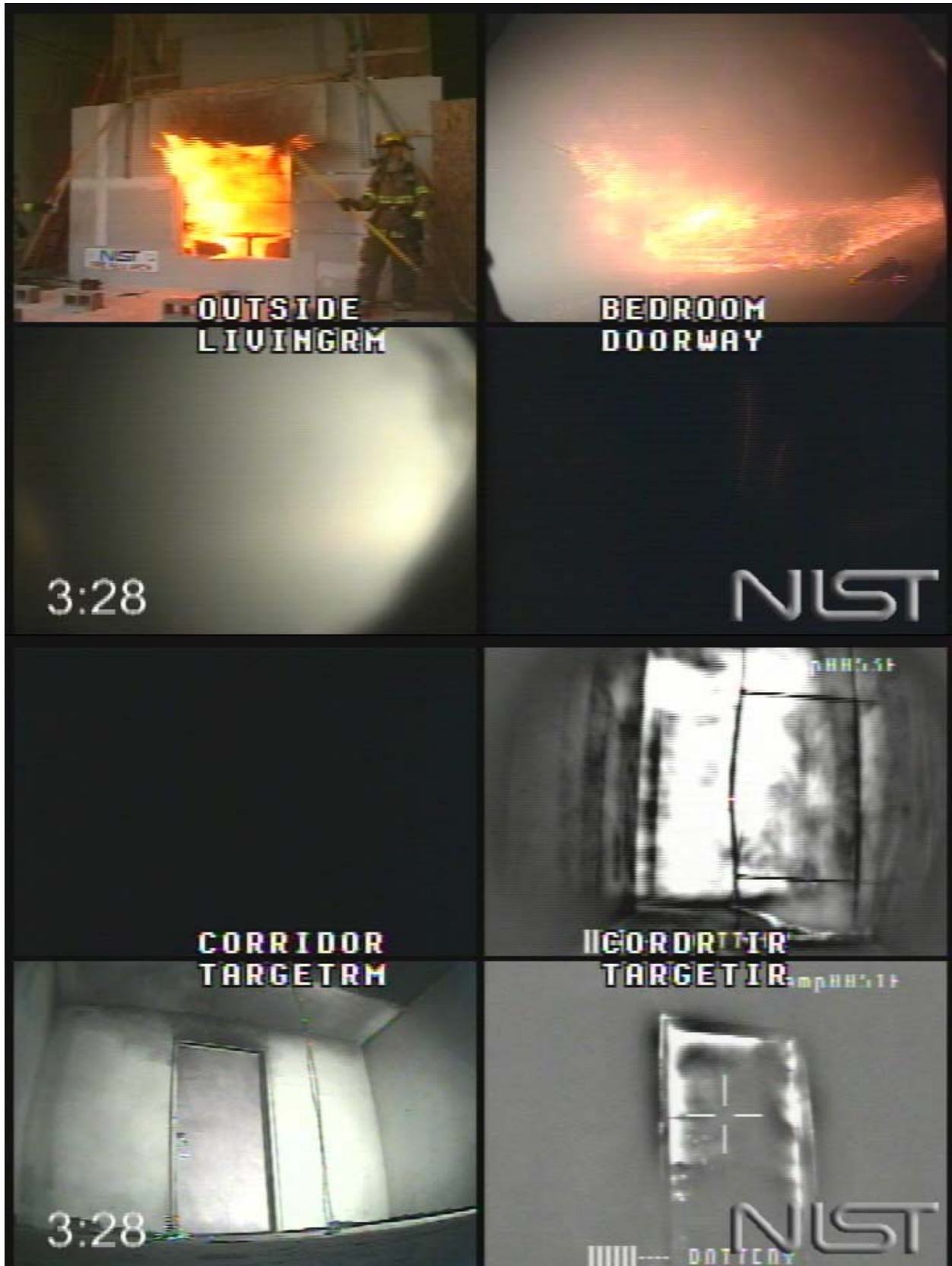
Figure 5.3.1-5. Experiment 3, window fully vented, 208 s after ignition.
