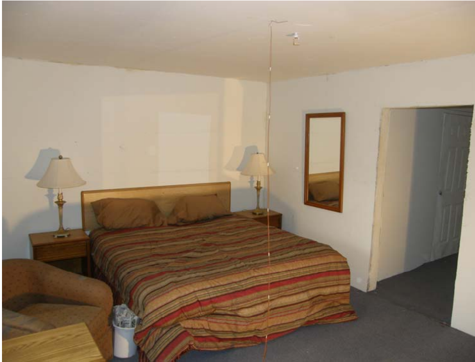
Figure 5-1. Photograph of the placement of the trash container fuel package ignition source.
