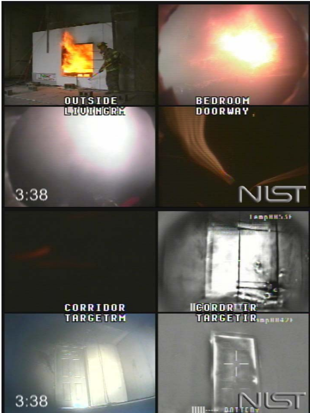
Figure 5.4.1-5. Experiment 4, window fully vented, 218 s after ignition.
