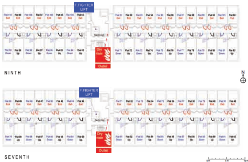
Fig 7: Layout of Shirley Towers showing the seventh (Bridgehead) and ninth (Fire) floors
