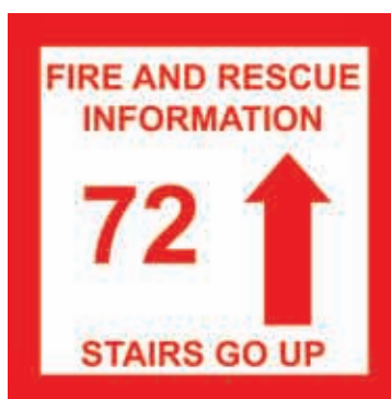
Fig 26: Diagram of flat marker denoting number and direction of entry (up or down).
